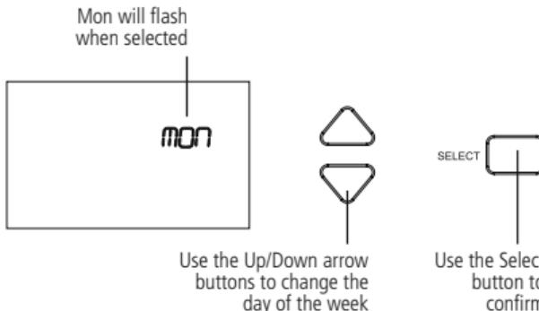
10.3 The P1 ON (Programme 1 ON) hour will flash, use the Up/Down arrow button to choose the hour and press the Select button once to confirm.
