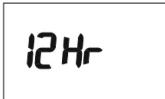
9.3 Use the Up/Down arrow buttons to either select 24Hr format, or leave it at 12Hr format, and then press the Select button once to confirm.
